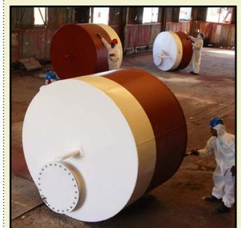
Mooring buoys being manufactured at FSHIL.
