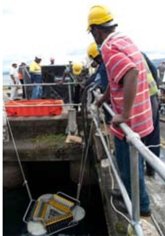
Participants lower a disc skimmer that will separate oil from seawater and pump the oil into inflatable tanks.
